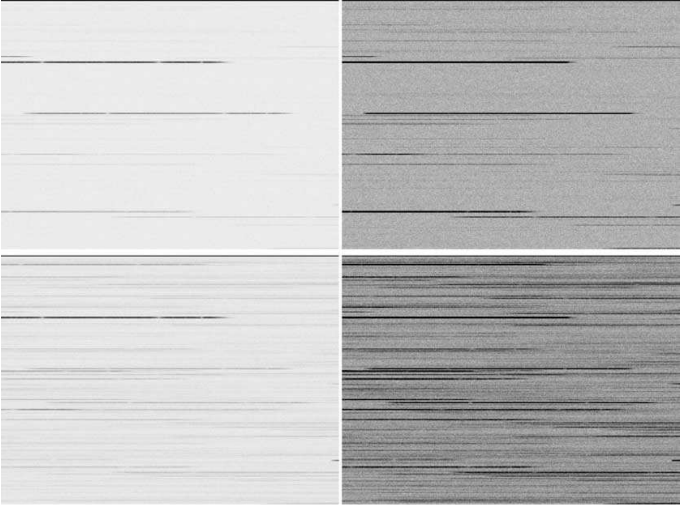
Figure 4. Simulated Gaia -RVS images for high Galactic latitudes (top) and |b| \leq 5^\circ (bottom), in linear scale (left) and in ‘thresholded’ linear scale (right). The images are generated for one transit of the focal plane of six CCDs, each with a readout noise of 2e^- .
